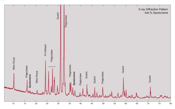
In most cases, automated mineralogy using QEMSCAN/MLA will be able to determine element deportment, however, it is not possible to detect Li by QEMSCAN/MLA due to the limitations of the XRF detector.
