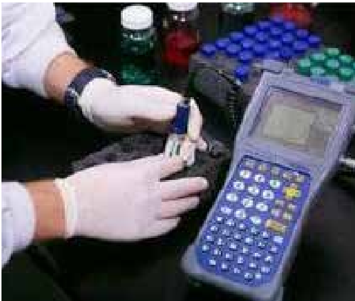
Figure 3 - Testing for the remaining useful life of a wind turbine gearbox oil
